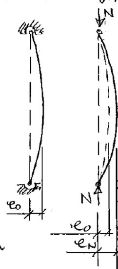
The magnitude of initial imperfection is much greater than the geometrical tolerances because the imperfection also accounts for the effect of residual stresses.
