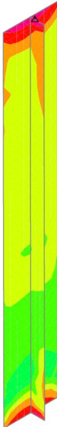
Figure 5-27: Calabria tower leg segment 17 plate A longitudinal strains due to the critical seismic load combination.
