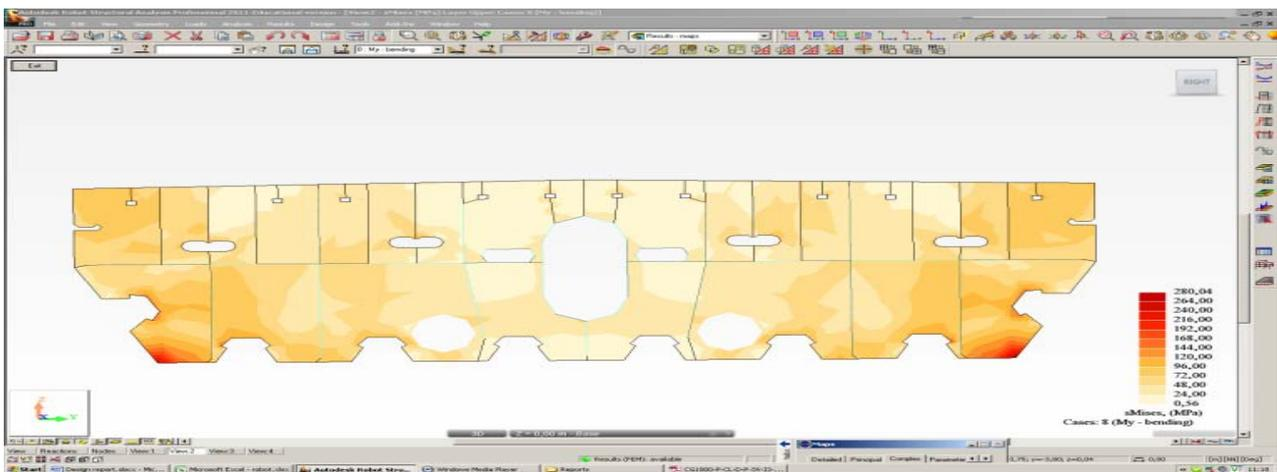
Figure 10-24 von Mises stresses, roadway girder diaphragm, case 12 (My+)
