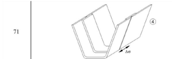
4. Point D represents the weld connecting deck plate to trough web. Being a partial penetration weld, an additional parasite bending moment becomes present due to the compression in the web of the trough and the eccentricity of the weld. This detail is only subjected to local effects. The weld corresponds to a detail category 71, see EN1993-1-9 Table 8.8, detail no.7.
