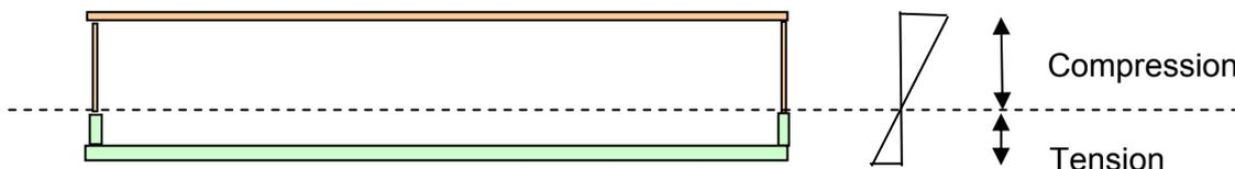
*Figure 7-3 Illustration of the assumption used for calculating effective properties for a bridge girder cross section (plates only)*
