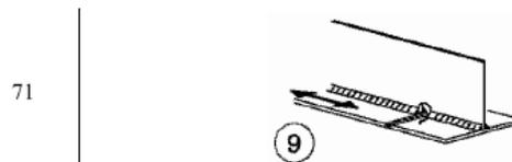
2. Point WB represents the top of the stiffener web connected to the either the main diaphragms or the intermediate diaphragms. Detail category 80, see EN1993-1-9 Table 8.4, detail no.8.
