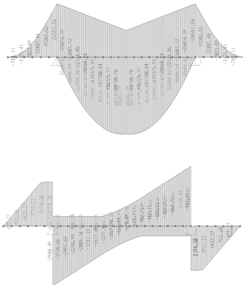
Figure 6-5: Forces induced by Load model SW/0
