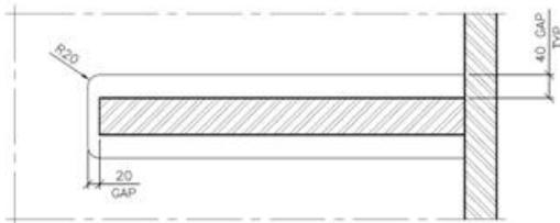
Figure 5-5 Current transverse diaphragm detail at longitudinal stiffener
