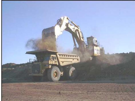
**Figura 4-9 Truck Loading: Overburden SCC 05-010-37**
