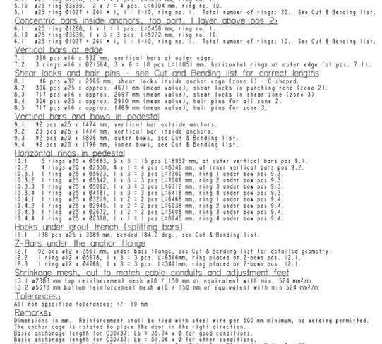
Number and height of C-shaped bars, shear locks and hair pins (see also Cut and Bending List)
