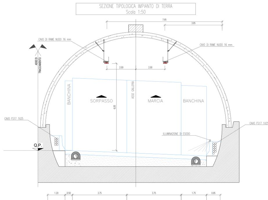
**PARTICOLARE MESSA A TERRA APPARECCHIATURE CLASSE I E MASSE METALLICHE**
