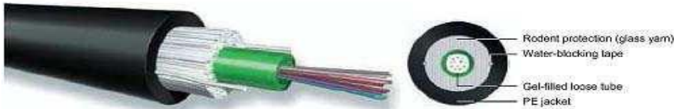
Figure 1: Fibre optic cable (cross section)
