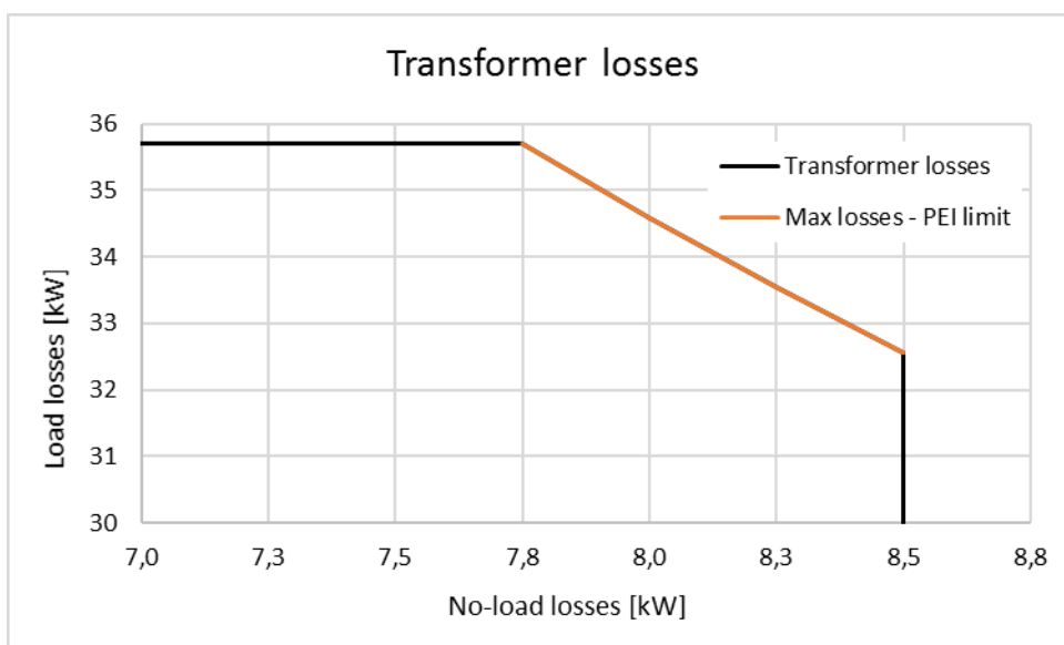
Figure 4-1 Transformer losses allowable area
