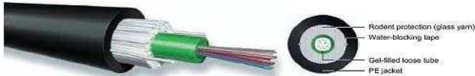
Figure 1: Fibre optic cable (cross section)
