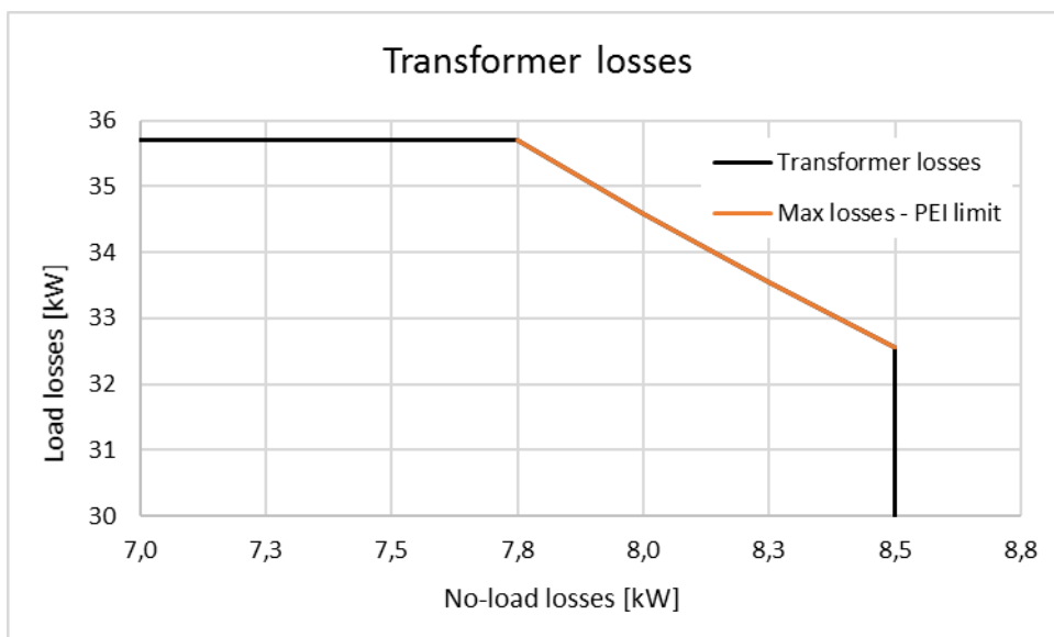
Figure 4-1 Transformer losses allowable area
