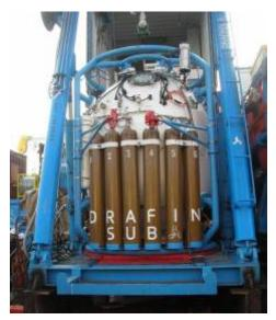
The Bell has a volume of 4.65 m<sup>3</sup> designed to bring 2 divers down to 200msw. It mates on the front side of the TUP chamber and take place on the dedicated A-Frame launch and recovery system. Since the system could be used with 6 divers under pressure, the SDC will be used as an additional evacuation unit.
