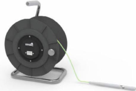
A piezometer consisting of a circular base and a long probe.                      |
