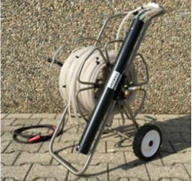
A portable pump on a metal frame with a wheel, used for sampling and dewatering. |
