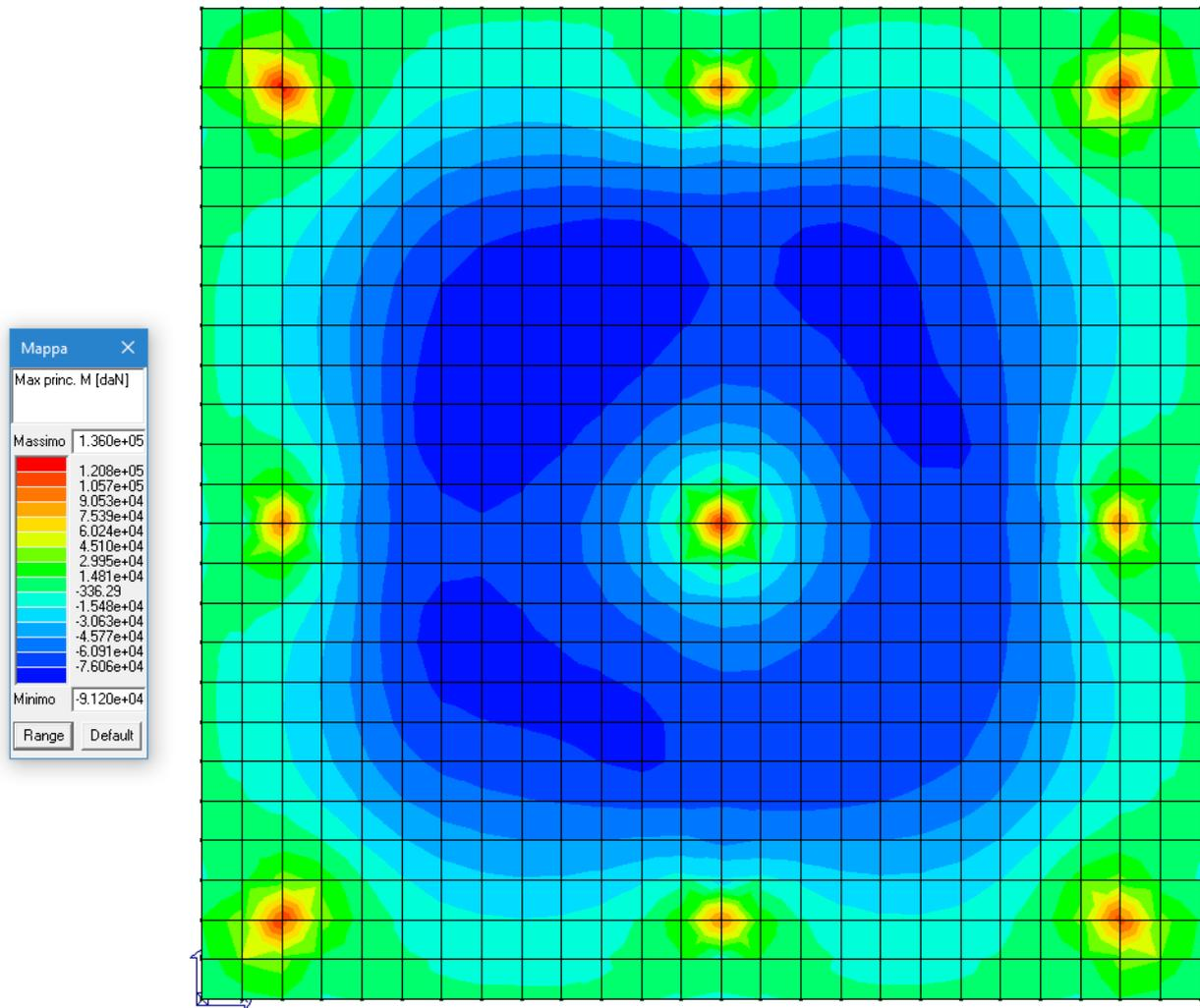
Figura 6 – Von Mises: Max princ. M (daN)
