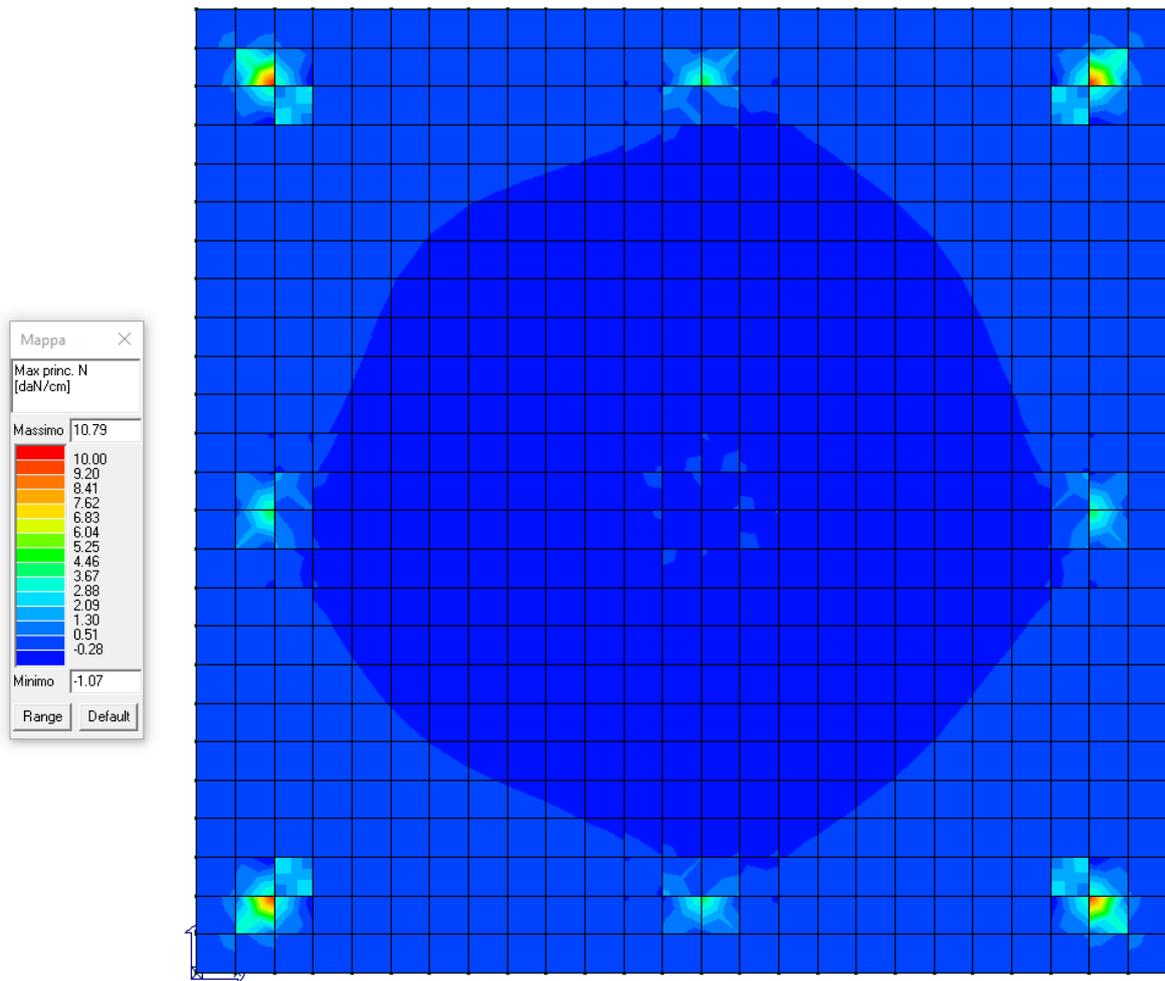
Figura 5 – Von Mises: Max princ. N (daN/cm)
