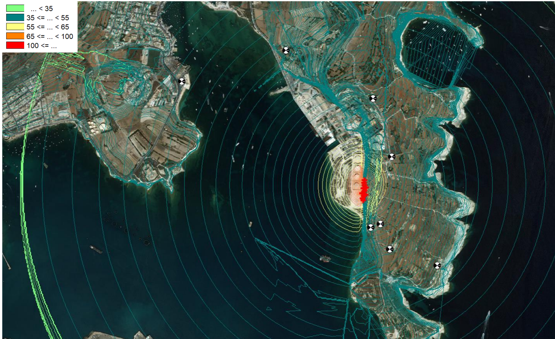
Figure 20: Construction Phase 1 – access construction road (all values in dB)
