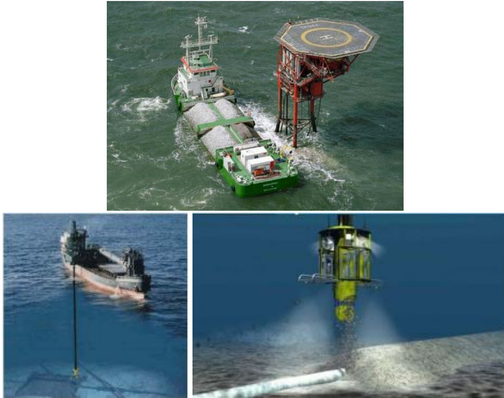
Figure 46: Different gravel-based pipeline support systems through the fall-pipe technology
