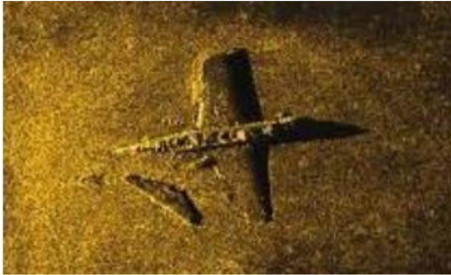
Figure 11: Metals reflecting acoustic pings from a plane wreckage (Source: McGowen & Morris, 2013)
