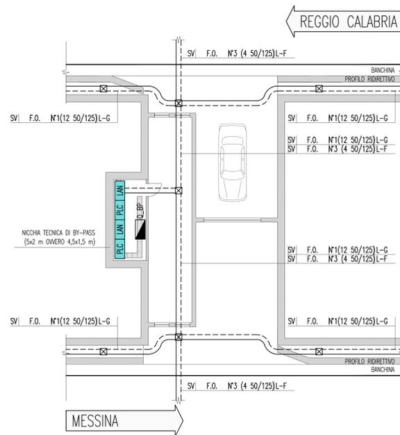
PARTICOLARE NODO RETE LAN/PLC DI BY-PASS
