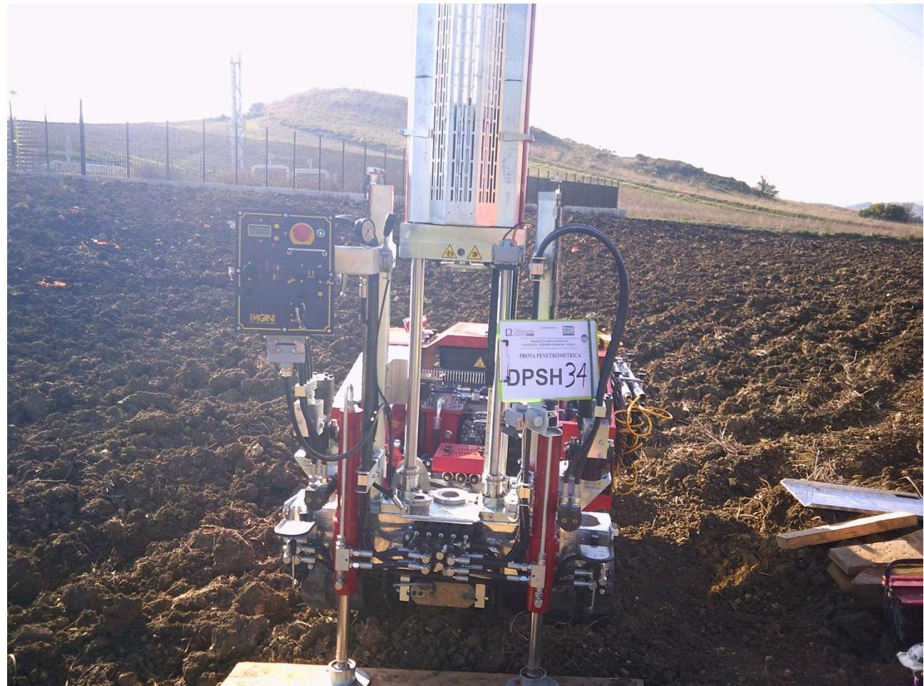
**PROVA PENETROMETRICA DINAMICA DPSH 34**
