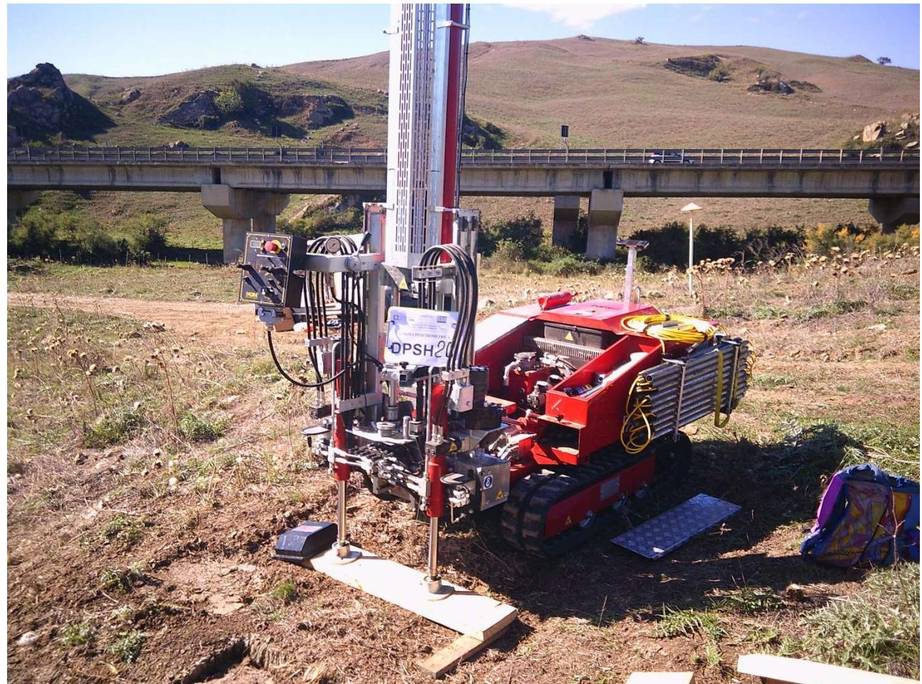
**PROVA PENETROMETRICA DINAMICA DPSH 20
