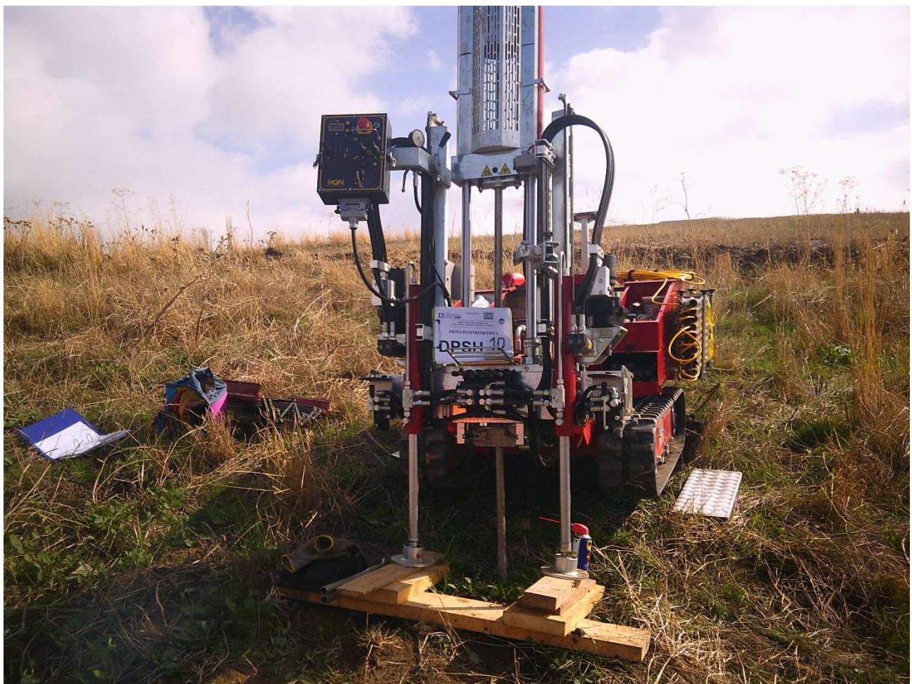
**PROVA PENETROMETRICA DINAMICA DPSH 10**
