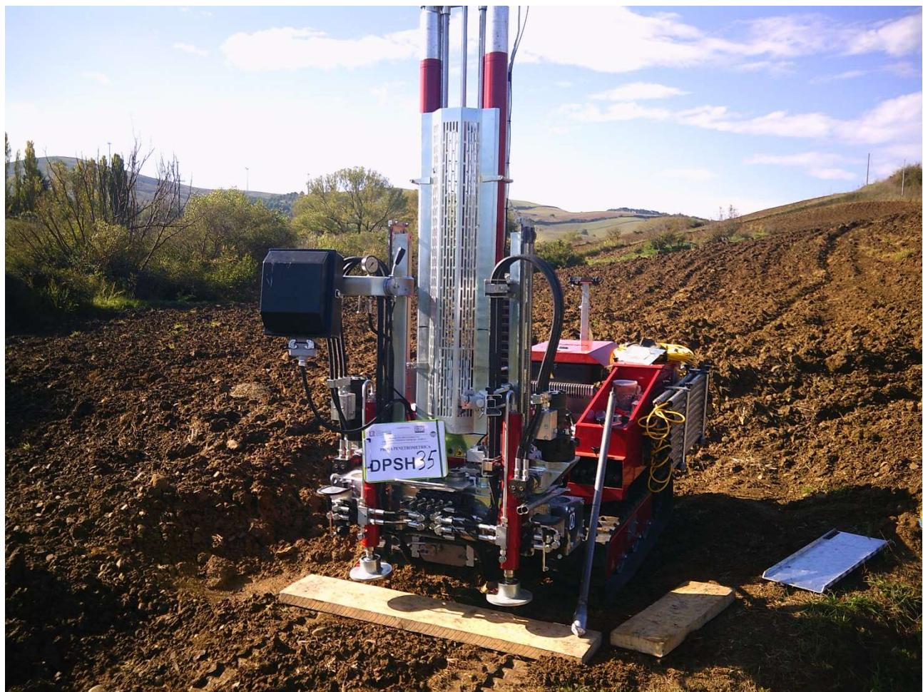
**PROVA PENETROMETRICA DINAMICA DPSH 35**
