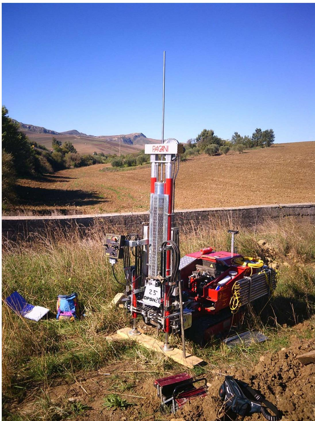
**PROVA PENETROMETRICA DINAMICA DPSH 25**
