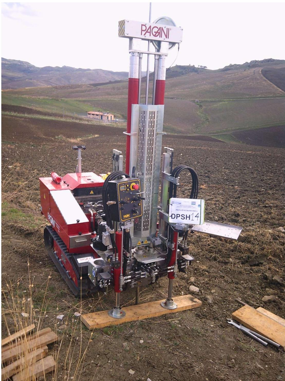
**PROVA PENETROMETRICA DINAMICA DPSH 14**
