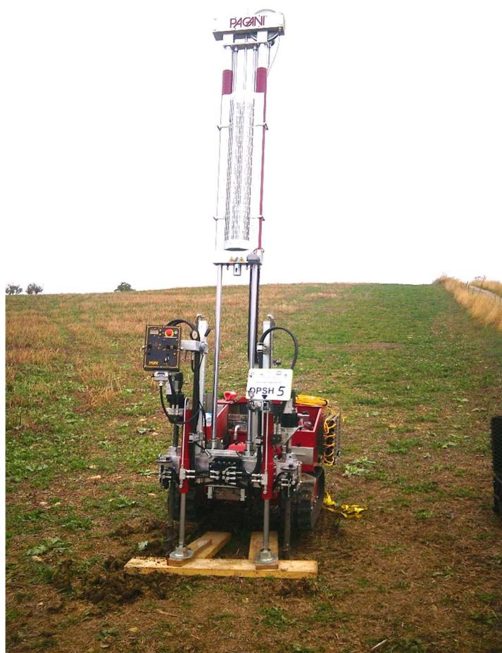
**PROVA PENETROMETRICA DINAMICA DPSH 5**
