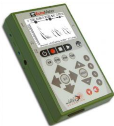
Bat detector ECHO METER EM3
