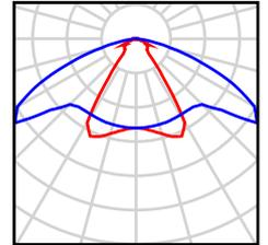
63 Pezzo ZUMTOBEL SLOT2 LED § 50 x CREE XT-E high power 90° - 70% dimm - mit opaler PM-Abdeckung - U=230V / P = 42.3W / Phi = 2110.0lm / T = 4158°K / x = 0.3772 / y = .3882 - I-Feld = cd/1000lm
