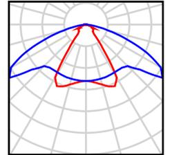
22 Pezzo ZUMTOBEL SLOT2 LED § 50 x CREE XT-E high power 90° - 70% dimm - mit opaler PM-Abdeckung - U=230V / P = 42.3W / Phi = 2110.0lm / T = 4158°K / x = 0.3772 / y = .3882 - I-Feld = cd/1000lm
