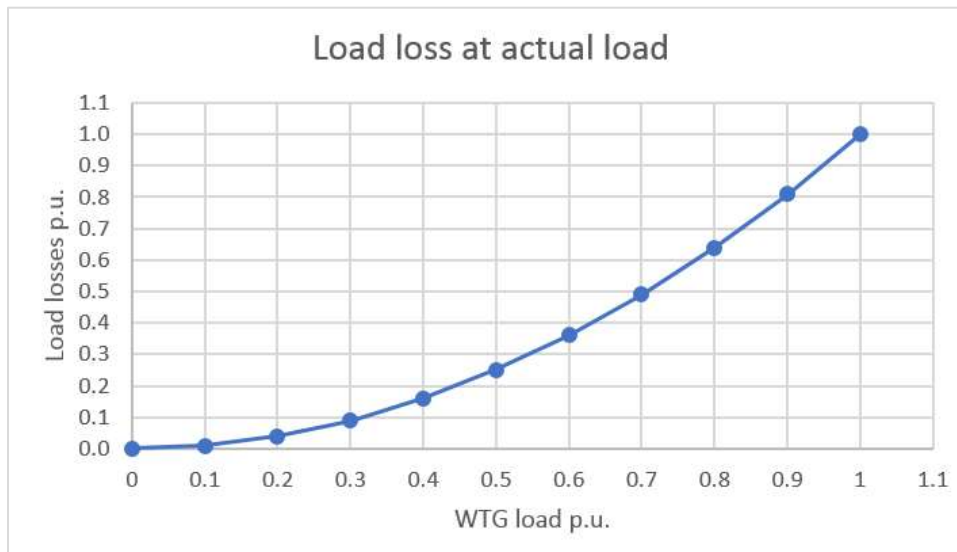
Figure 4-2- Transformer load losses scaling.
