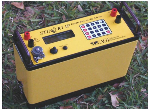
Figura 2 – Resistivimetro “STING R1/IP”
