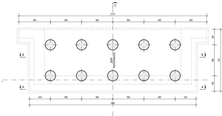
Figura 7: Pianta carpenteria\_Spalla 1
