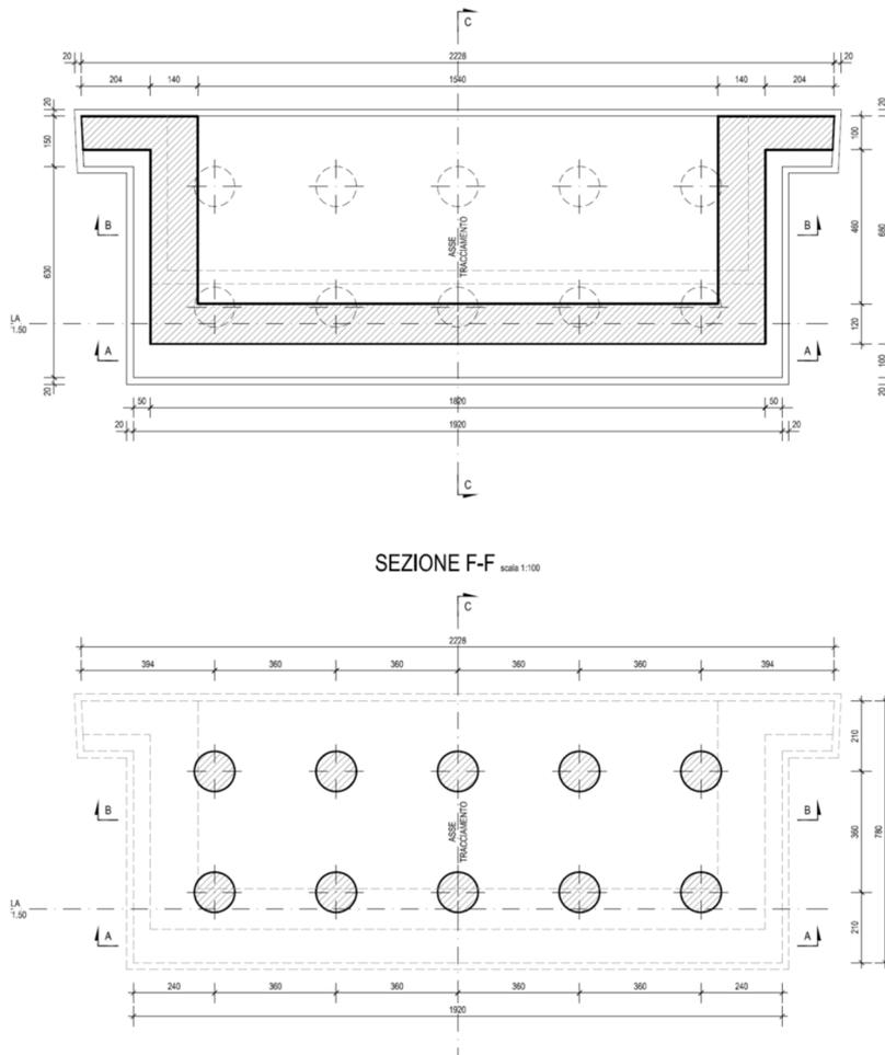
Figura 7: Pianta carpenteria\_Spalla 1
