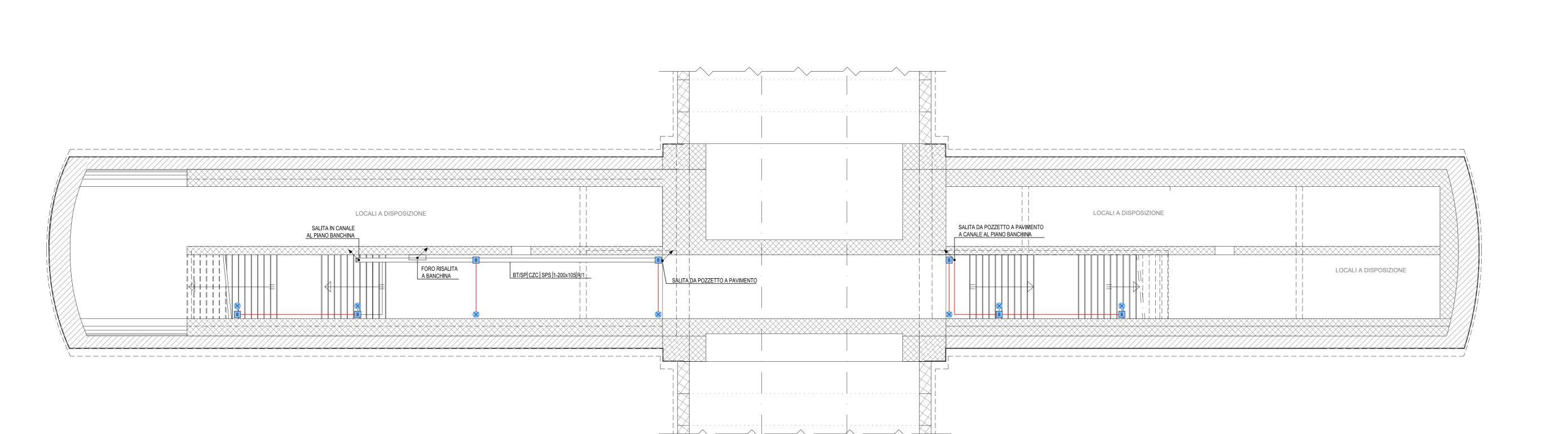
FINESTRA PEDONALE F3 bis: IMPIANTI FM-LUCE PIANTA PIANO SOTTOBANCHINA (SCALA 1:100)
