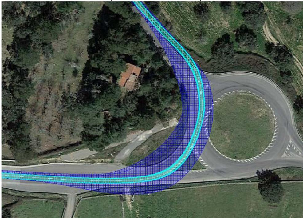
Turn left on the roundabout. Enlarge road on the north side (otherwise we have problems with the steering of the dolly). Remove electricity pole in the south. Little oversail on private property.
