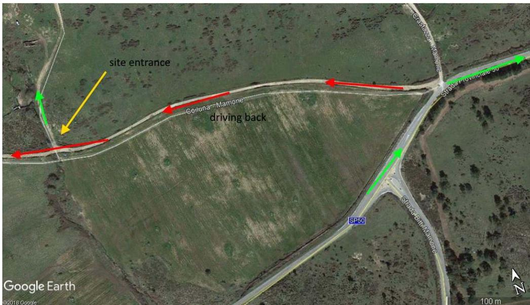
Possibility to reach site entrance: drive on SP 50, reverse on Strada Coiluna-Mamone, enter the site. All roads in the windfarm must be designed according to GE Specification for Site Roads and Crane Pads
