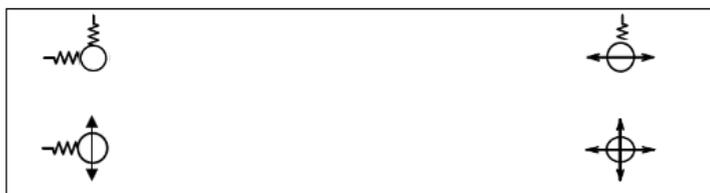
Figura 10. SCHEMA APPOGGI
