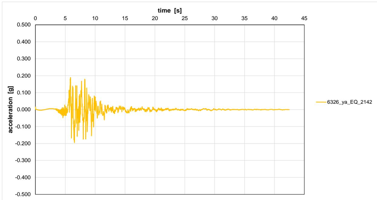
Figura 7 – Accelerogramma naturale: Waveform ID=6323, Earthquake ID=2142
