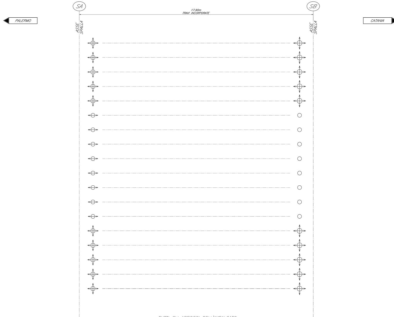
TUTTI GLI APPOGGI DELL'IMPALCATO A TRAVI INCORPORATE SONO DEL TIPO A DISCO ELASTOMERICO CONFINATO
