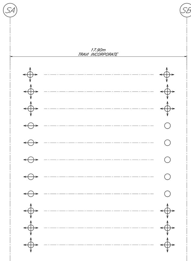
TUTTI GLI APPOGGI DELL'IMPALCATO A TRAVI INCORPORATE SONO DEL TIPO A DISCO ELASTOMERICO CONFINATO
