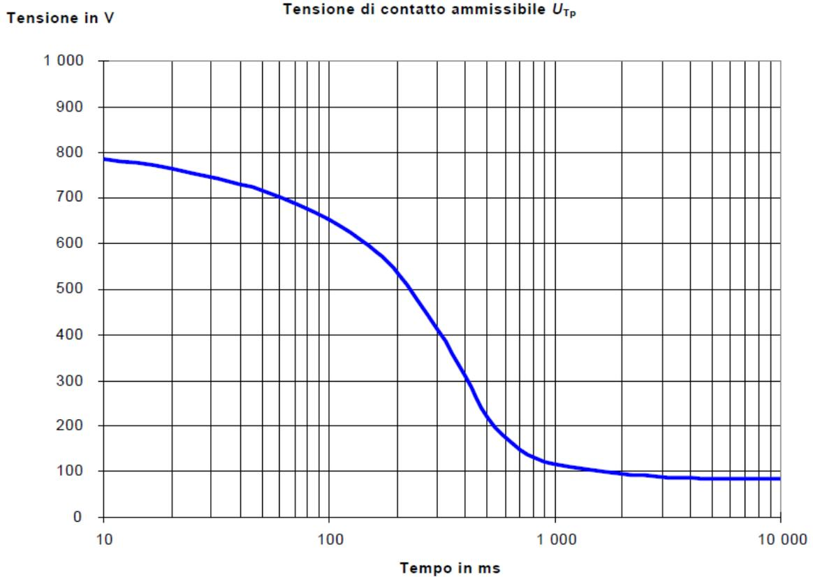
Figura 4 – Curva Tempo-Tensione (Norma CEI EN 50522 § 5.4.3)
