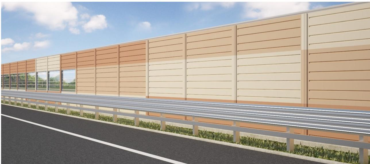
**FIGURA 7-3 – BARRIERA ACUSTICA OPACA FONOASSORBENTE SU RILEVATO – VISTA LATO SORGENTE**
