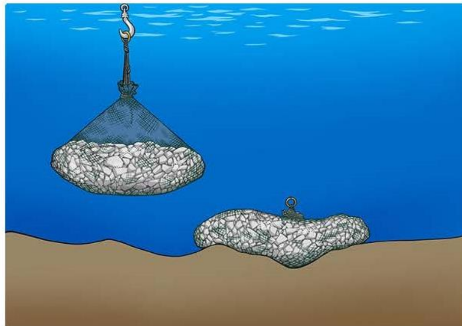
Filter Unit fits even with uneven seabed without gaps.
