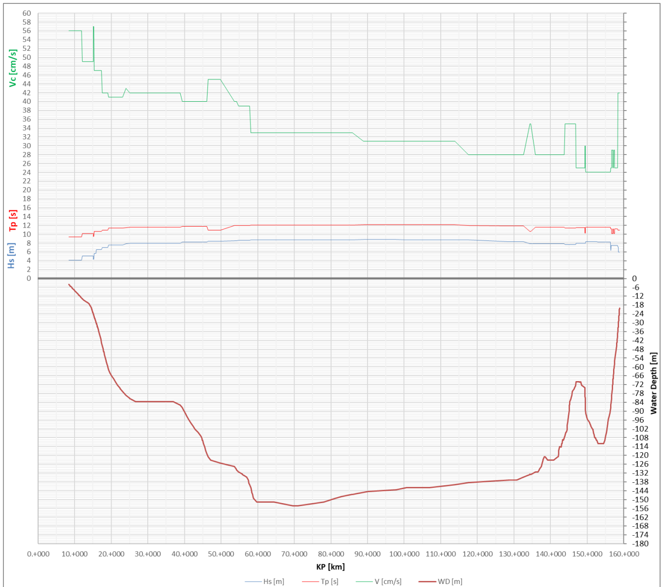
Figure 4 – Offshore Section – Waves and Currents Distribution (Omni)
