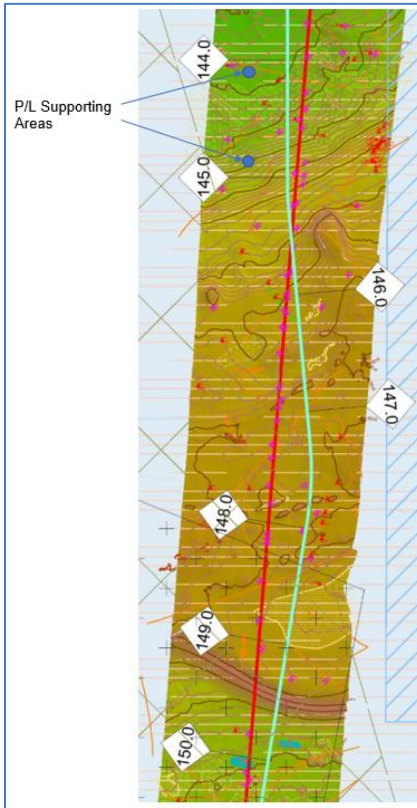
Figure 4.36 – P/L Supporting – Uneven Seabed from KP 144.1 to KP 144.8
