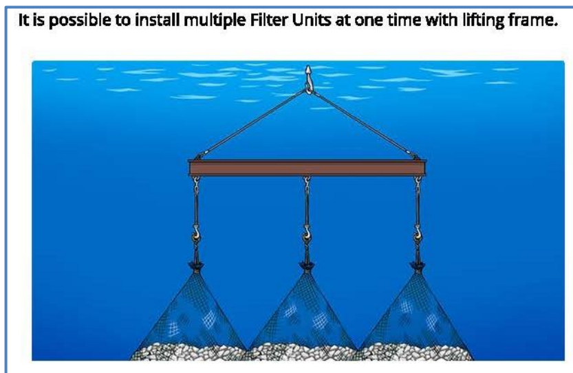
Figure 4.6 - Rock Filter Unit – Example of Multiple Installation Technology
