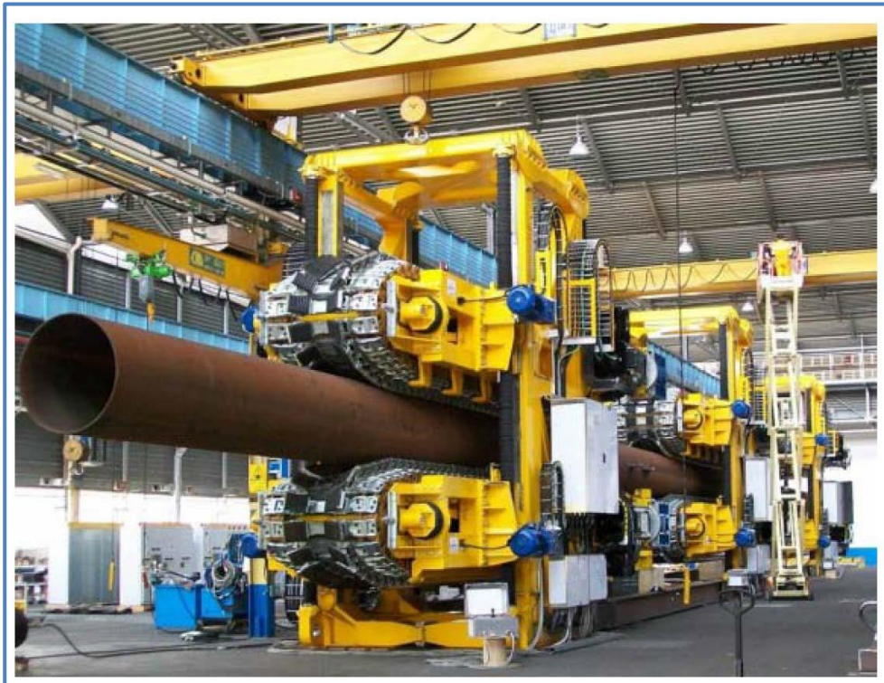
Figure 4.12 – S-lay Vessel – Typical Tensioner Arrangement
