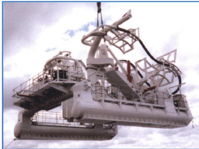
Figure 4.19 - Post-trenching Works – Example of Jet Sled Equipment
