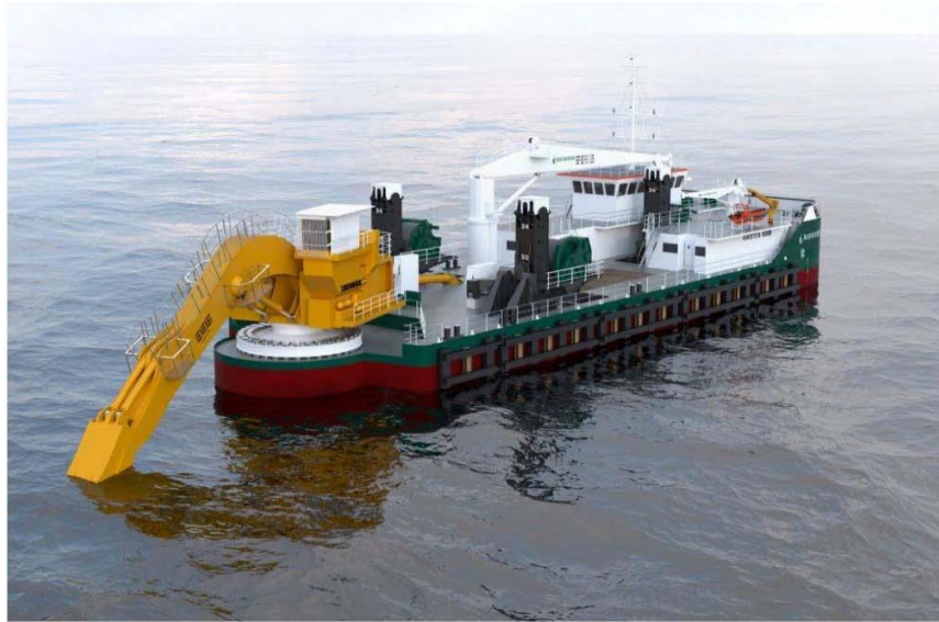
Figure 4.3 – Preparation Works at HDD Offshore Bore Hole Exit - Example of Backhoe Dredger
