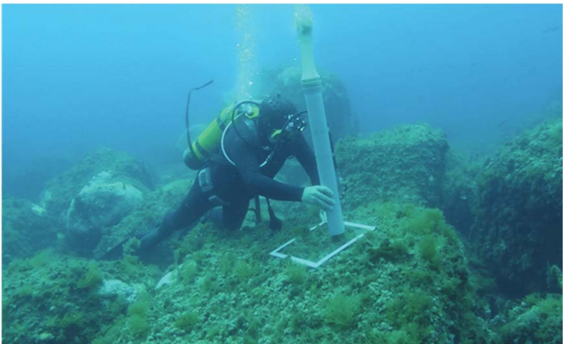
Figure 8. Diver making use of an air sorbena on rocky assemblages
