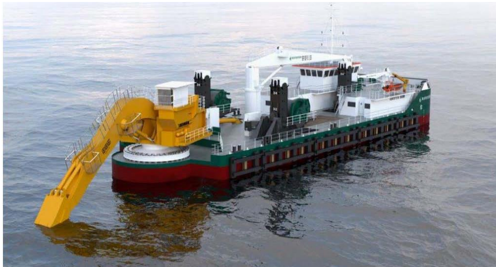
Figure 13: Preparation Works at HDD Offshore Bore Hole Exit - Example of Backhoe Dredger
