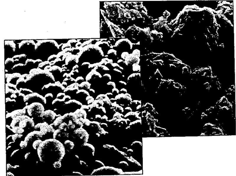
Figure 3. Fly ash (left) and portland cement (right).
