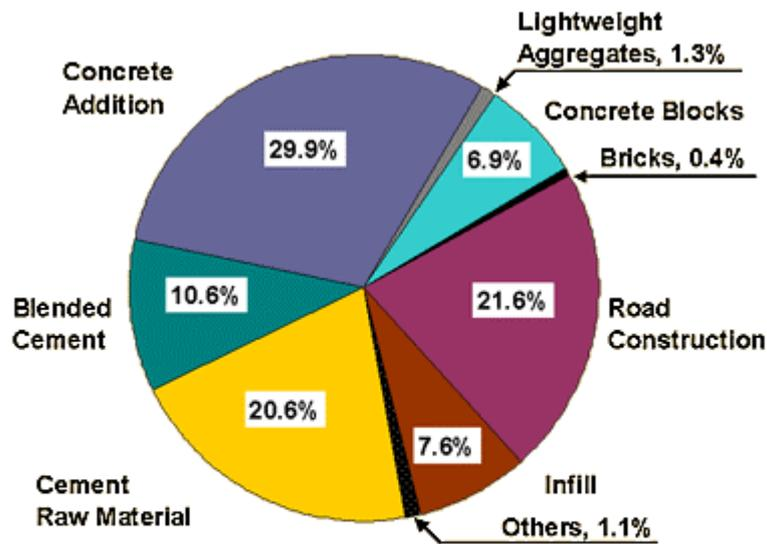
**Figura 4 - Utilization of Fly Ash in the Construction Industry and Underground Mining in Europe (EU 15) in 1999**
