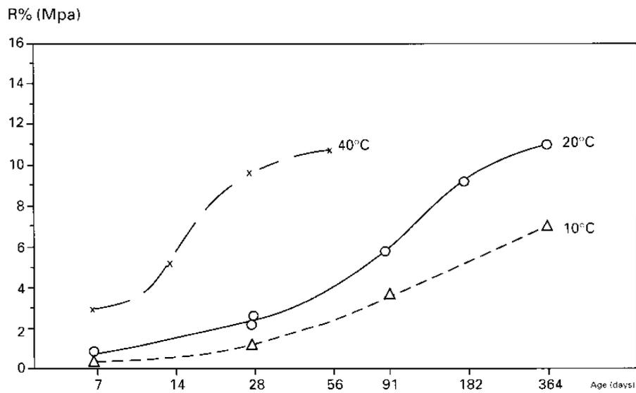
Figure 1. Development of the unconfined compressive strength of GFA.
