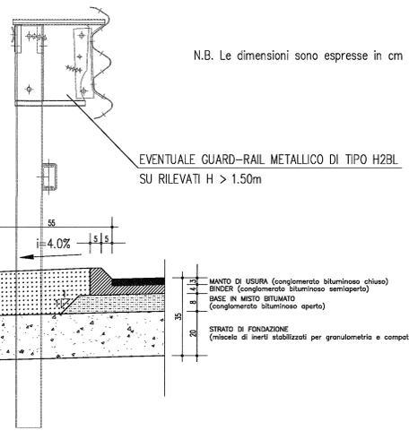
STRADA TIPO F2 – SEZIONE TIPO IN RILEVATO (H < 1.50m)
