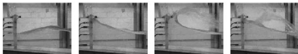
Fig. 16.18. A sequence showing the function of a parapet/wave return wall in reducing overtopping by redirecting the uprushing water seaward (back to right).
