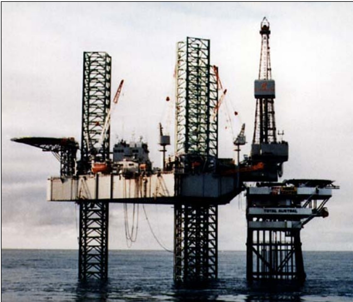
Fig 1 impianto Jack-Up Drilling Unit (tipo "GSF Key Manhattan")
