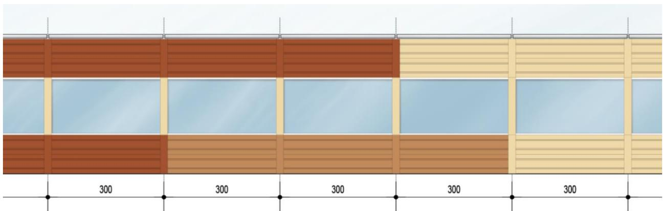
FIGURA 5-7 – BARRIERA ACUSTICA MISTA FONOSSORBENTE-FONOSOLANTE – PROSPETTO LATO SORGENTE
