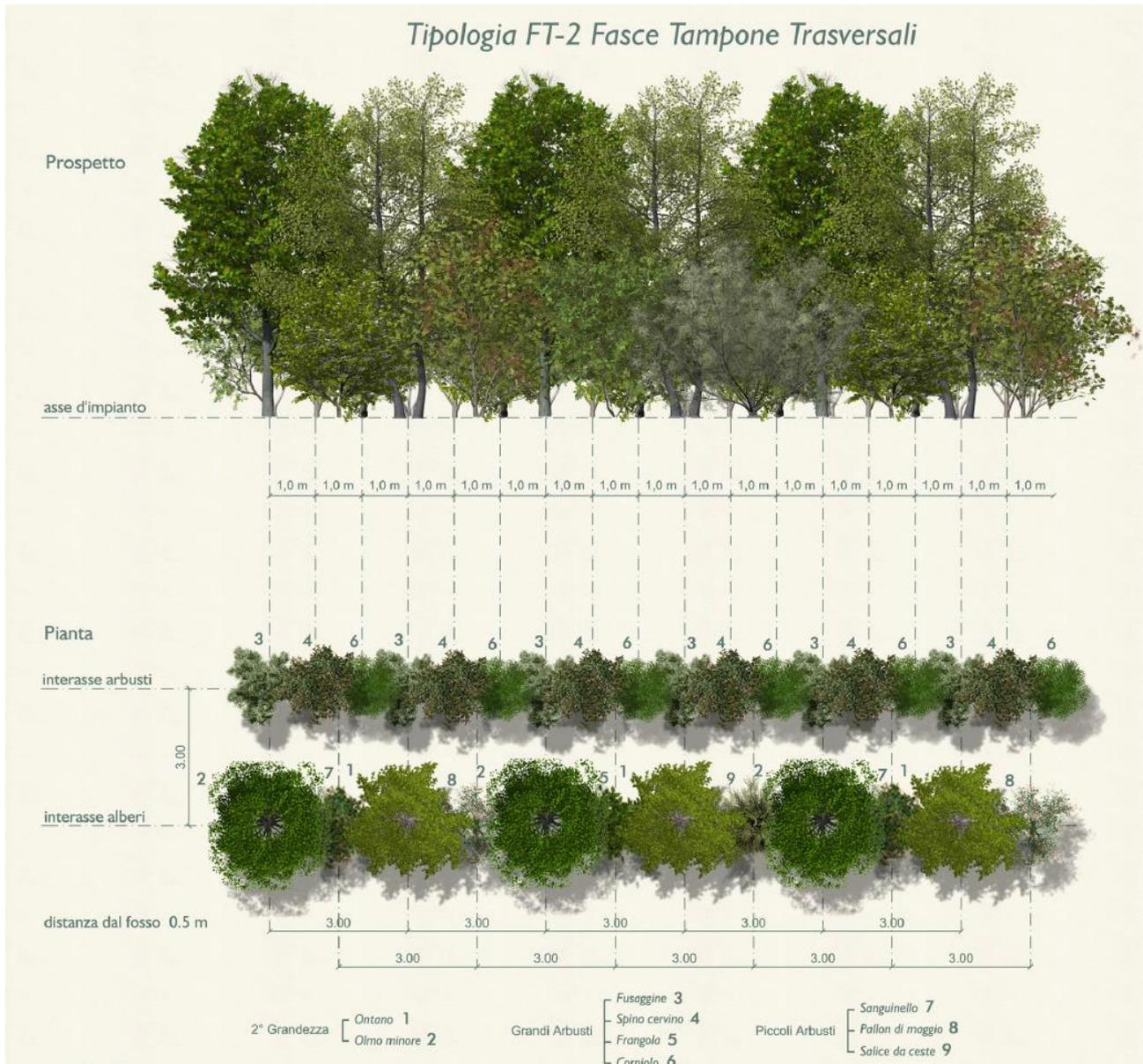
FIGURA 4-45 - TIPOLOGIA FT2 : FASCE TAMPONE TRASVERSALI
