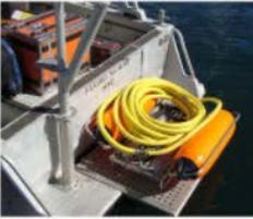
The Geo-Source 200 L is also compatible with the standard cable (40 mm<sup>2</sup> plus 4 x 10 mm<sup>2</sup>) used for the Geo-Source 200 and 800
