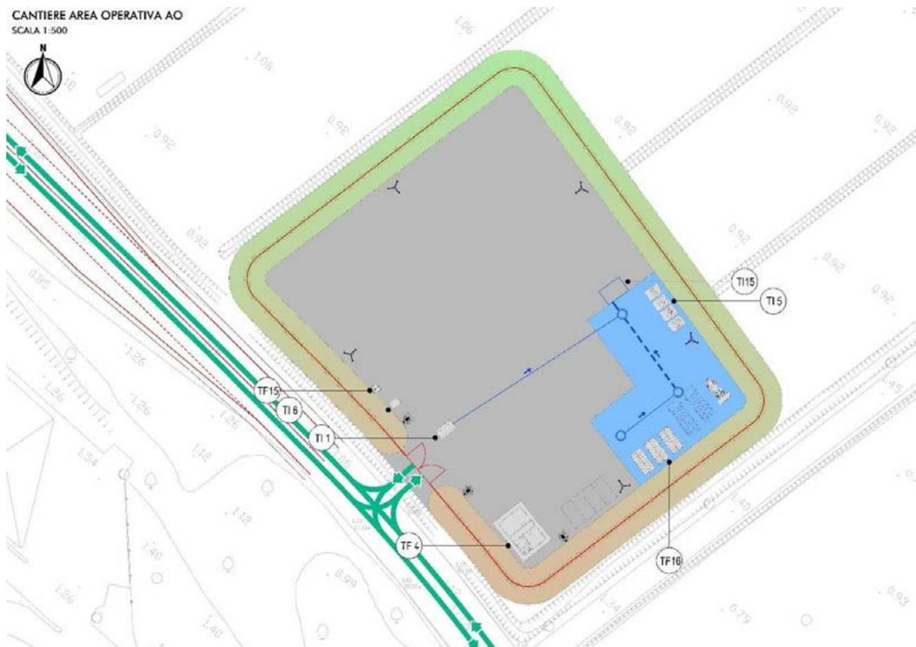
**FIGURA 6-19 LAY-OUT FUNZIONALE DEL CANTIERE AO (ESTRATTO DALL'ELABORATO T00IA10CANLF01)**
