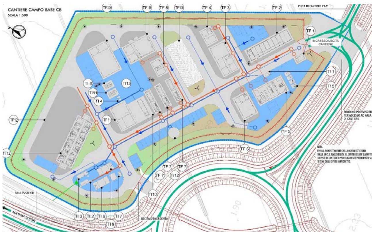
FIGURA 6-8 LAY-OUT FUNZIONALE DEL CANTIERE CAMPO BASE "CB" (ESTRATTO DALL'ELABORATO T00IA10CANLF01)
