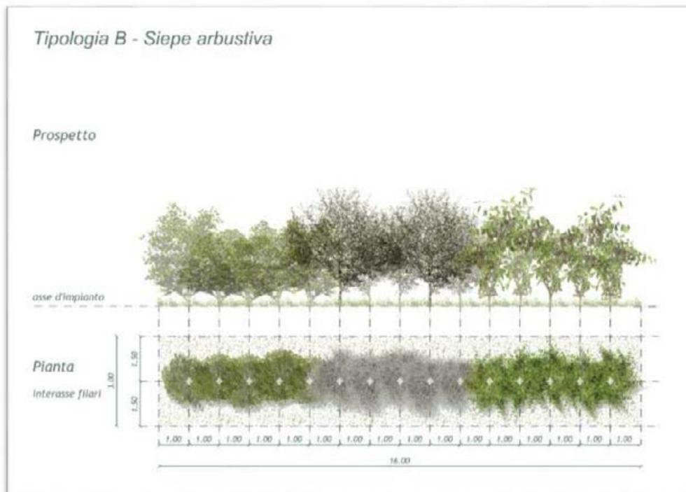
**FIGURA 10-46 SCHEMA ASSOCIATIVO DI IMPIANTO RELATIVO ALLA TIPOLOGIA B**
