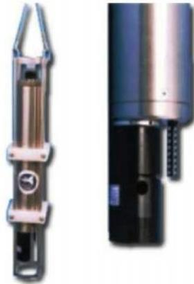
The CTD600 Mk 3 is a self-recording Conductivity, Depth and Temperature unit (CDT) with a high accuracy and large memory capacity. The fish can be connected directly to a P.C using a current-loop converter, or to a surface display unit which can then be connected to a P.C. Various additional sensors can be fitted to give temperature, pressure and conductivity.
