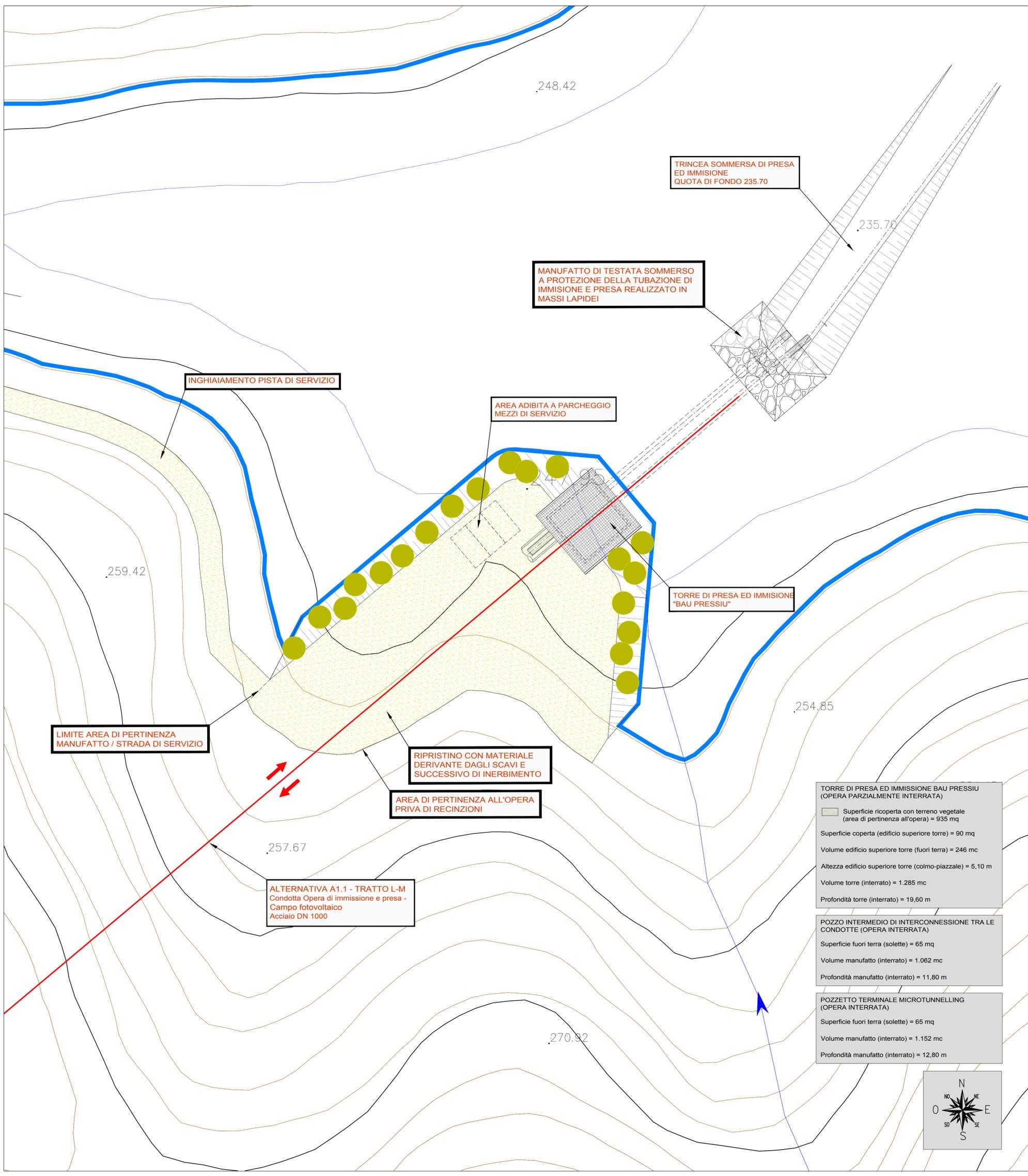
**TORRE DI PRESA ED IMMISSIONE BAU PRESSIU (OPERA PARZIALMENTE INTERRATA)**
