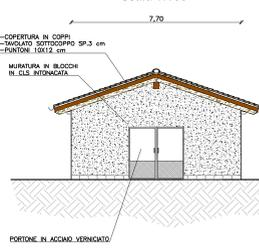
**OPERA DI IMMISSIONE E PRESA LAGO BAU PRESSIU PROSPETTO NORD-OVEST**
