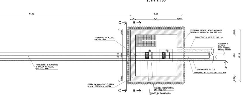
**OPERA DI IMMISSIONE E PRESA LAGO BAU PRESSIU PROSPETTO SUD-OVEST**
